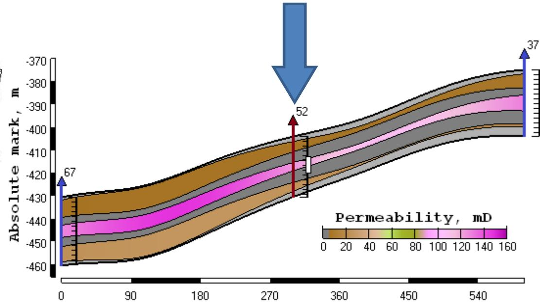
Isolation of the production well perforation interval
