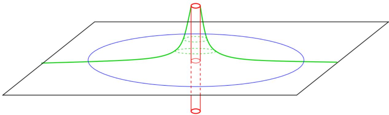
Radial flow pressure field with near-well singularity.
