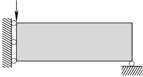
Figure 1: The design domain, boundary conditions, and external load for the optimization of a half MBB beam.
