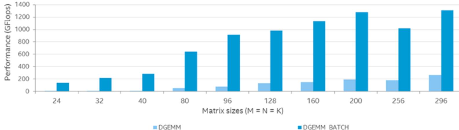
Configuration info - Versions: Intel® Math Kernel Library (Intel® MKL) 2017; Hardware: Intel® Xeon Phi™ Processor 7250, 68 cores (34MB L2 cache, 1.4GHz), 96 GB of DDR4 RAM and 16 GB MCDRAM; Operating System: RHEL 7.2 GA x86\_64;
